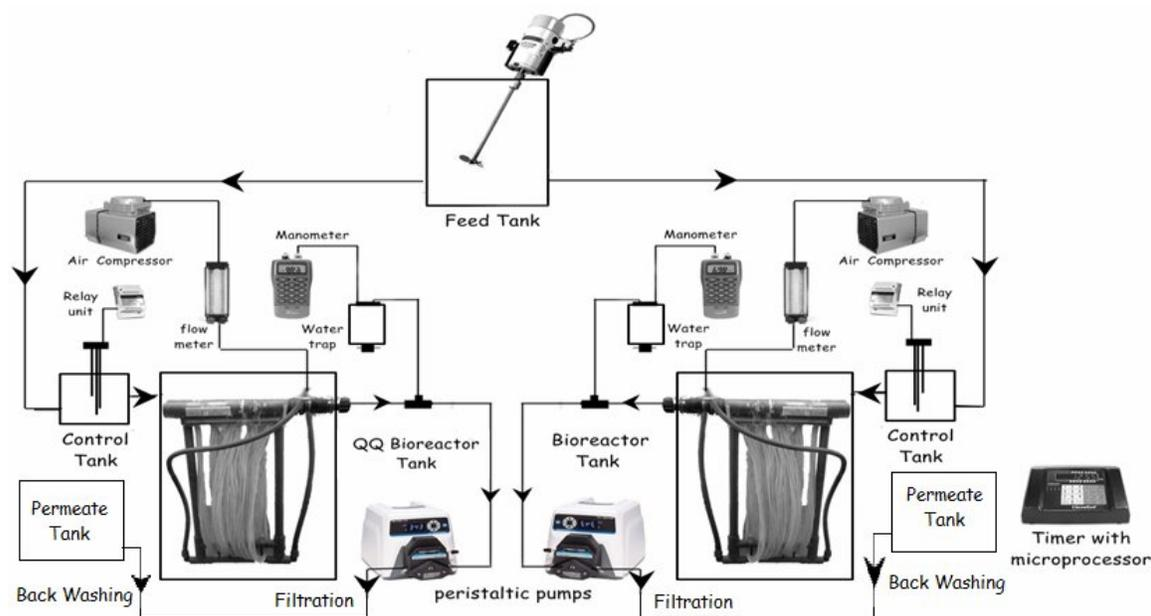
Fig. 1: Schematic of semi-pilot scale C-MBR and QQ-MBR systems with backwashing.
